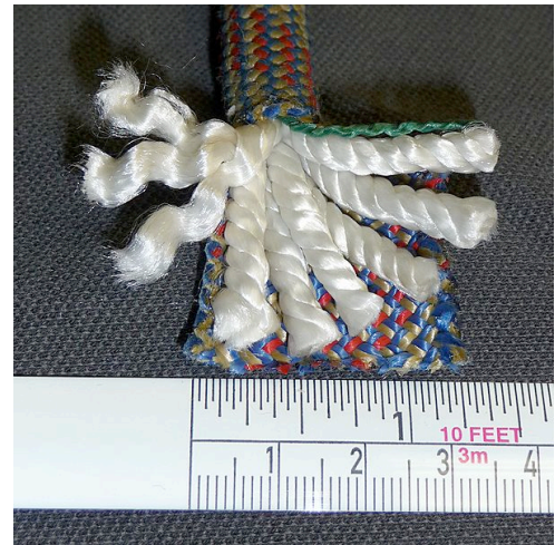
Figure 7.4.18. Twisted rope, made up of seven three-ply yarns. In the picture, the three plies of the left-most core yarn are spread apart (upload.wikimedia.org/wikipedia/commons/1/1a/Kernmantle_climbing_rop_e_dynamic_Sterling_10.7mm_internal_yarns_and_plyes.jpg).
