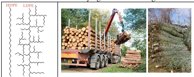
Figure 7.4.11. Schematic of the polymer stacking in HDPE versus LDPE (left) and the analogous stacking of logs versus branched trees (pics: logs trees http://www.northerngrid.org/ngflwebsite/chopwell/images/photographs/log_stack.jpg ; and http://www.istockphoto.com/file_closeup/nature/4814662-christmas-trees-fresh-cut-pile-stacked.php?id=4814662 ).
